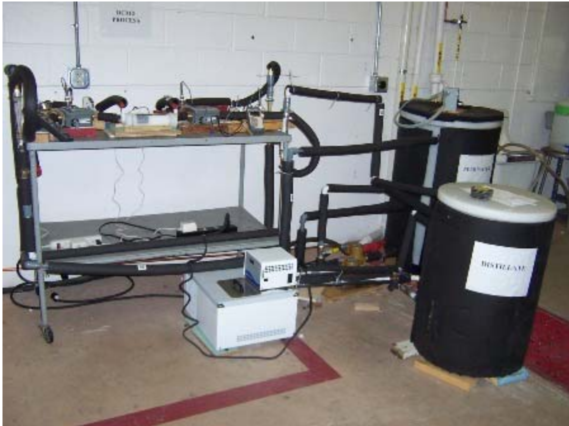
Figure 6. A Complete View of DCMD Application by Using Hollow Fiber Membrane Module
