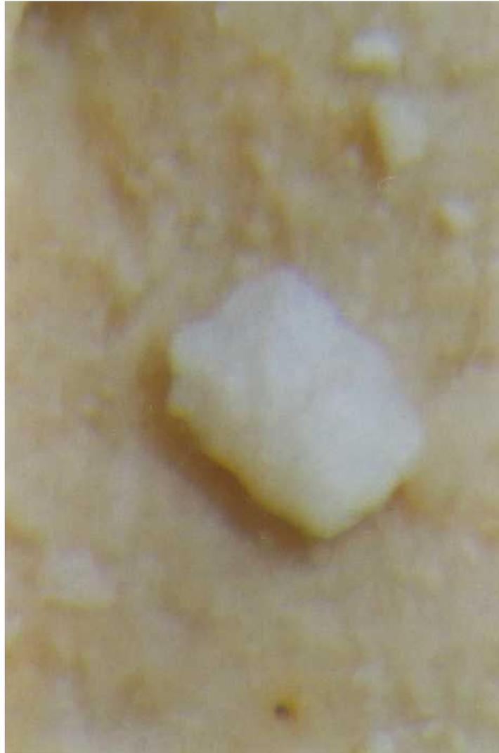
Figure 7. Microphotograph of crystal observed on kaolinite membrane at conclusion of Experiment 7. The size of this crystal is about 0.025 mm by 0.0275 mm and the total magnification is 2000X.
