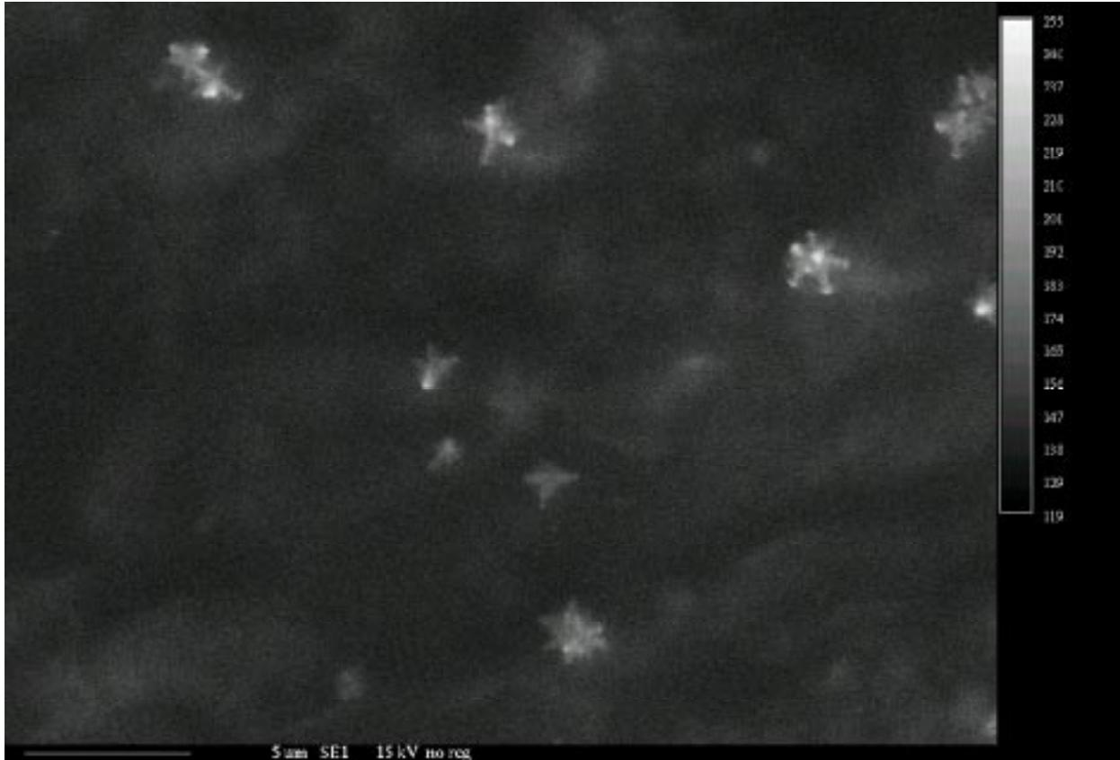
Figure 18. Electron micrograph of unknown crystals on surface of membrane from Experiment 14. These crystals do not have the habit of NaCl crystals. No energy dispersive X-ray scan is available for these crystals. Their composition is unknown. No similar crystals were observed on any of the other membranes.
