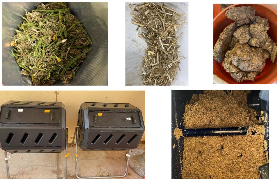
Figure 1. Initial compost materials and composters: (top from left to right) hemp leaves, hemp stalks, and cow manure; (bottom from left to right) tumbling composters, compost after three days
