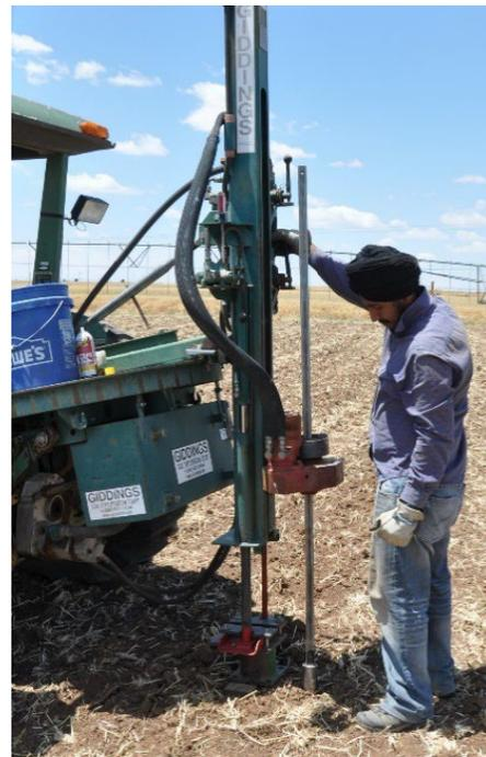
**Figure 3.** Installation of neutron access tubes in the study area.
