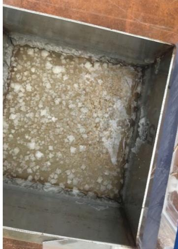
**Figure 6. Picture showing of salts precipitated in the metal basin during solar distillation**
