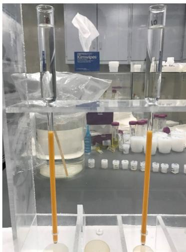
**Figure 12. Separation of REEs from PW concentrate using cation exchange chromatography (effective column length 7.75 inch and a cross-sectional area of 0.5 cm<sup>2</sup>).**
