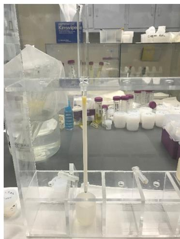
**Figure 13. Individual separation of La, Nd and Eu from the combined REE using HDEHP chromatography (white column).**
