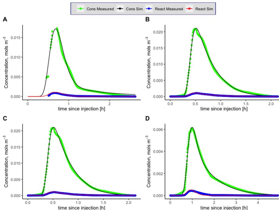
**Figure 2.** Tracer BTCs of measured (dotted) and best models fit simulations (lines) based on the transient storage model for A) N injection, B) NC injection, C) NP injection, and D) CNP injection.
