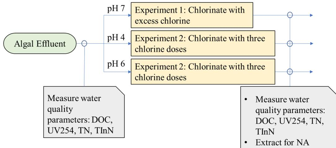
Figure 1: Schematic diagram of the experimental plan
