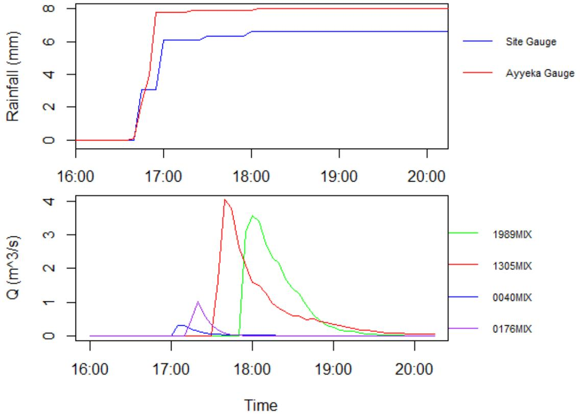
Figure 1: Rainfall Hyetograph and Discharge Hydrograph for flow event on 10/2/2018
