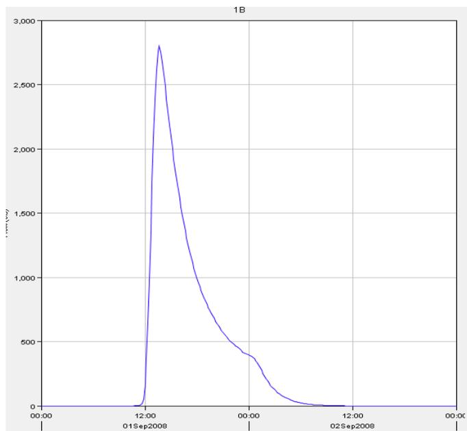
Fig 9. Hydrograph from 2<sup>nd</sup> simulation (Snyder's)
