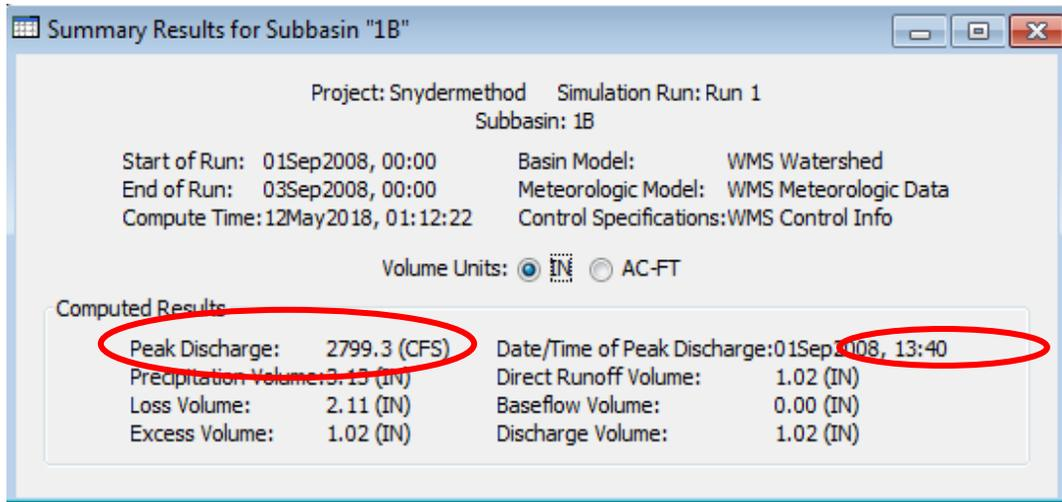
Fig 8. Snyder's method outputs
