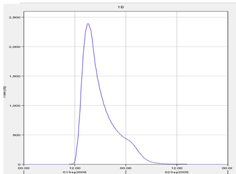
Fig 7. Hydrograph from 1<sup>st</sup> simulation (SCS-CN)
