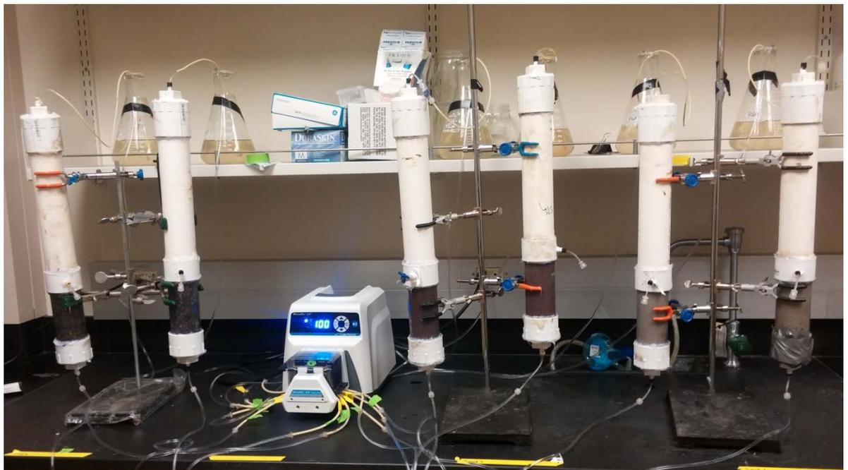
Figure 3. Experimental set up. Laboratory tracer test experiments
