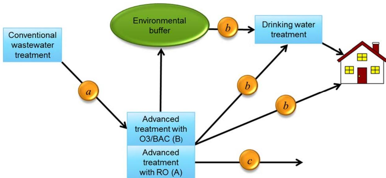
**Figure 2. Pumping and piping flow paths considered with the hypothetical reuse scenarios in this paper. Flow path a takes the WWTP effluent to the site where both the advanced treatment and the environmental buffer will be located; path b moves the effluent from advanced treatment or the environmental buffer to the DWTP influent or the distribution system, which are practically in the same location; and path c takes the RO concentrate to disposal wells.**
