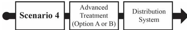
**c. Scenarios 4A and 4B are the same as 3A and 3B, respectively, except that the drinking water treatment plant is omitted prior to distribution.**
