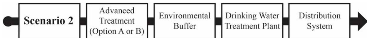
**a. Scenario 2 includes conventional plus advanced wastewater treatment (2A includes RO and 2B includes O<sub>3</sub>/BAC), followed by discharge to an environmental buffer, withdrawal, and drinking water treatment.**
