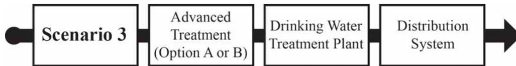
**b. Scenarios 3A and 3B are the same as 2A and 2B, respectively, except that the environmental buffer is omitted.**
