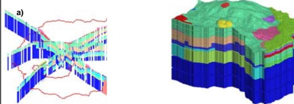
Fig. 3(a-b). To develop a finite element mesh, we digitized 400 pseudoboreholes (a) into geographic coordinates. Then we used Leapfrog Hydro to interpolate geologic volumes at unknown locations from these boreholes. Finally, the geologic model developed by Leapfrog Hydro is used to assign hydraulic properties to each node in a mesh for the Redondo Creek watershed of Valles Caldera (b).
