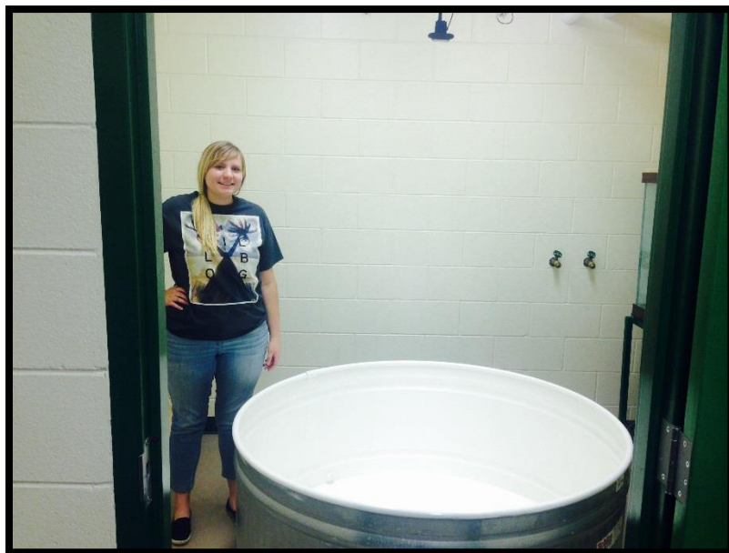
Image 1: Graduate student researcher, Sabrina Michael, stands next to her experimental observation room. The 1.5m galvanized steel tank, painted with white epoxy paint, is centered underneath the camera for tracking.
