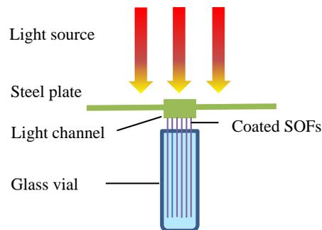
Figure 1. Batch photoreactor with catalyst-coated SOFs
