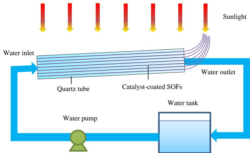
Figure 2. Continuous-flow photoreactor with catalyst-coated SOFs
