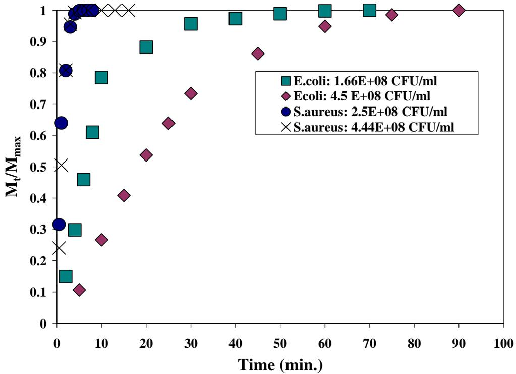
**Figure 1.1** Fractional uptake curve of *E.coli* K12 and *S.aureus* SH 1000 on SWCNT aggregates
