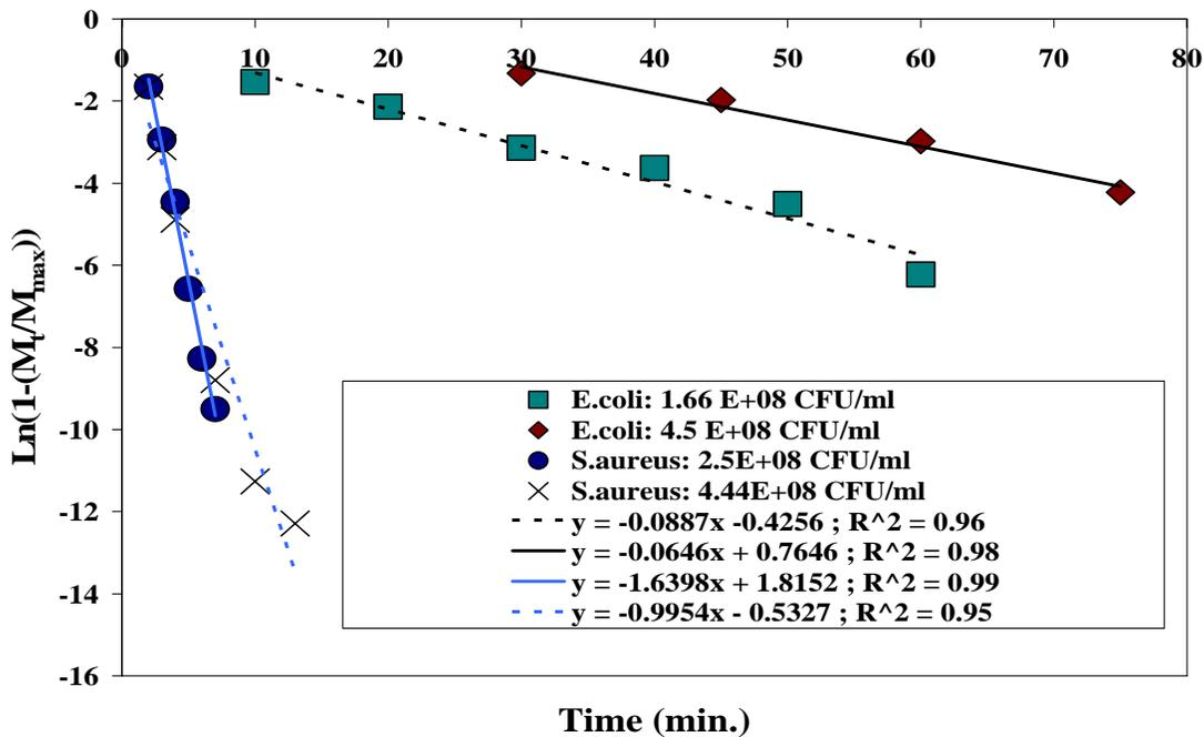
**Figure 1.2** Correlation of adsorption kinetics data with diffusion model for *E.coli* K12 and *S.aureus* SH 1000 on SWCNT aggregates at 25°C
