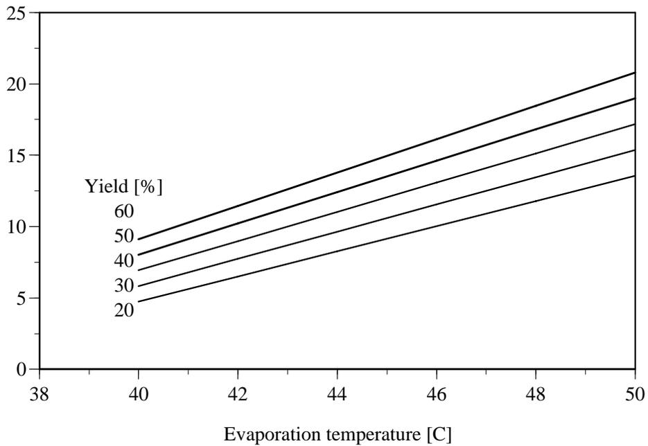
Figure 2. Relationship between PV array area/evaporator area, product yield, and evaporation temperature
