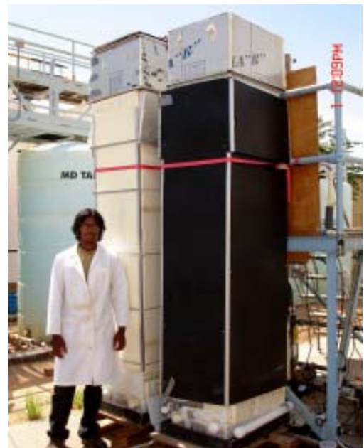
Prajwal Vikram is working with the Dewevaporation Process for Brackish Water Desalination.
