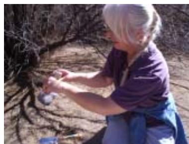
*April Ulery taking a salinity measurement of a soil sample in the field.*
