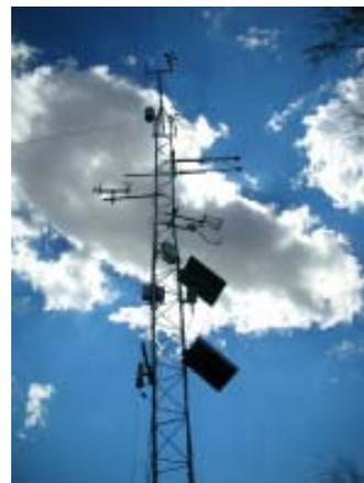
*One Propeller Eddy Covariance (OPEC) system installed at Bosque del Apache to measure evapotranspiration (ET).*
