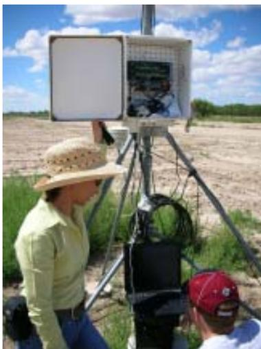
*Data logger at the tower (Bosque del Apache) collecting ET and climate data at 30-minute intervals.*
