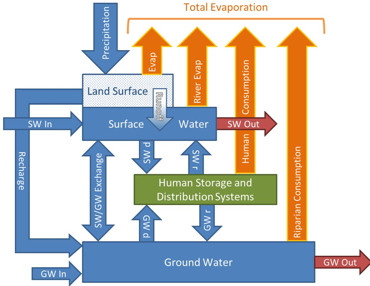
Figure 3 Conceptual water balance diagram.
