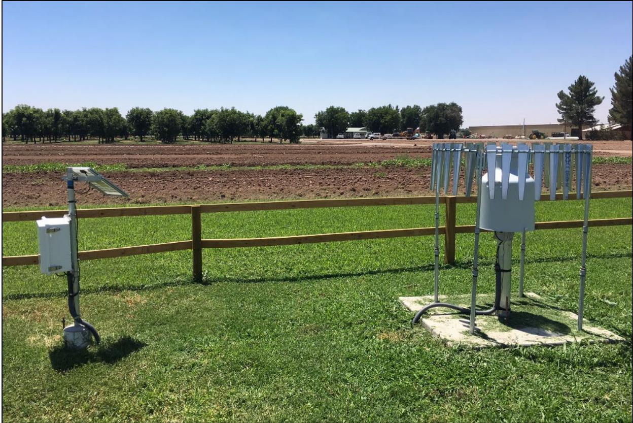
Figure 5. Pluvio rain gauge with wind shield
