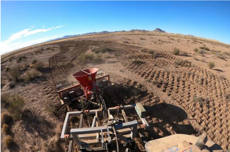
The Seed hopper distributes seed before the imprinter rolls the ground (HDNP et al., 2022)
