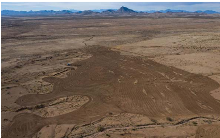
The imprinter rolls the land, creating water-harvesting divots in the surface (HDNP et. al, 2022)
