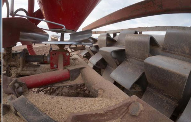
Detail of seed hopper (HDNP et al., 2022)
