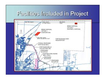
Project features being considered and evaluated according to the National Environmental Policy Act (NEPA) include two concentrate disposal locations and methods (evaporation ponds vs. deep well injection) and three potential plant locations.
