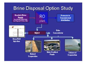
A brine disposal option study was implemented in the early phases of the project because the brine disposal investigating, permitting, and construction requirements represented the critical path for the project schedule. The options being considered can be immediately implemented technologically. Certainly, there are many other options that might be considered, but they are project specific.
