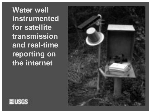
Figure 15. Water well instrumented for satellite transmission and real-time reporting on the internet.
