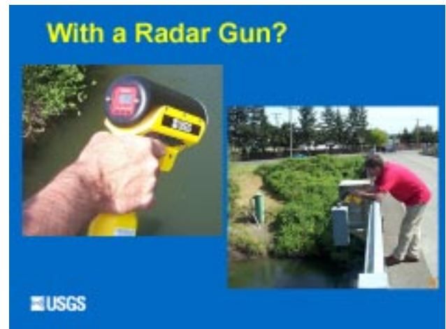
Figure 12. Radar guns are used to measure surface velocity.
