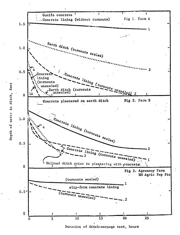
the seepage rate in a nearby earth ditch from which water was leaking through unsealed turnouts. A comparison of curves 1A and 4 shows a rate of water loss from the lined ditch to be greater than the loss from the unlined ditch.
