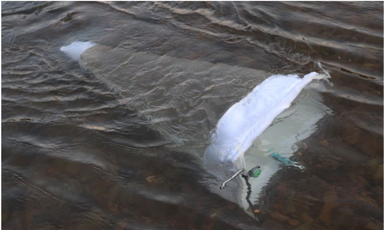
Figure 4. Example of a drift net deployed at the Bosque Redondo (BR) field site. Each net was fitted with a mechanical flow meter to quantify filtered volumes.
