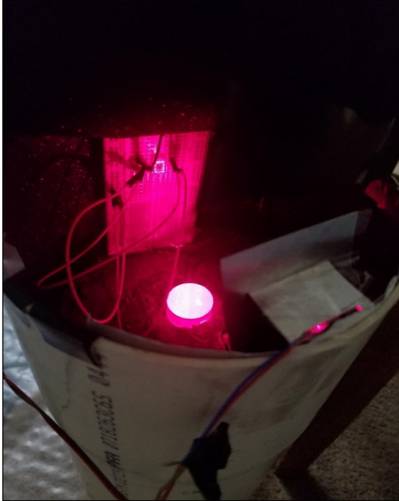
Figure 5. Plexiglas rod inserted in a soil column with an attached light emitter.
