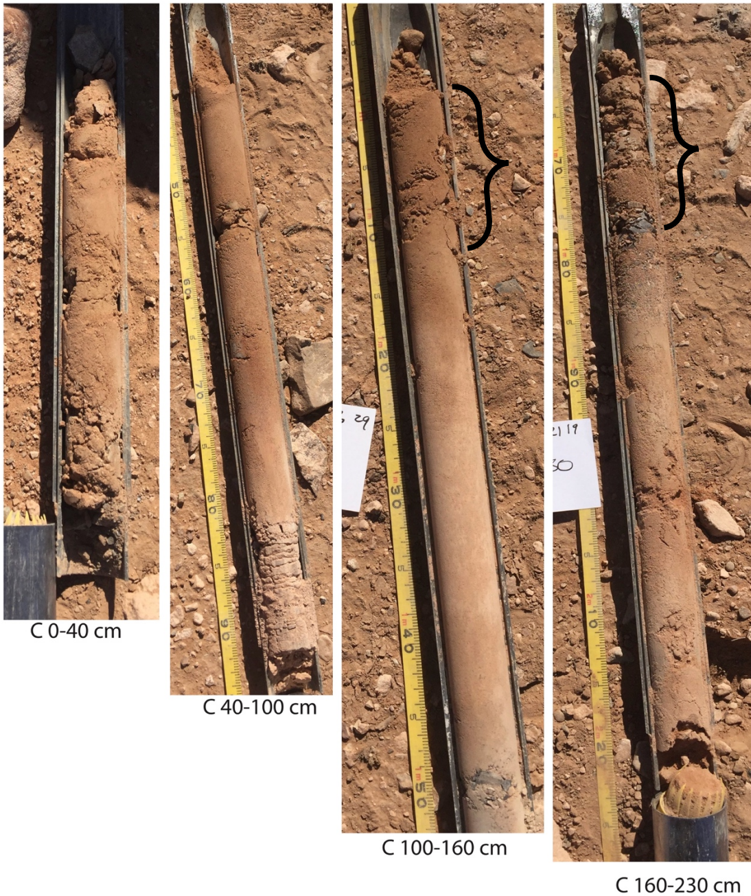
Figure 9. Photos of the first four core barrels extracted from Channel C. The depths used to label each core are the uncorrected depths, which do not match perfectly with Figures 4-7. The black braces indicate portions of C100-160 and C160-230 that have low chloride and may be sediment fallen from above.
