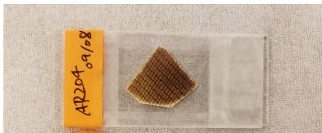
Figure 6. A Prepared Membrane Sample for CLSM
