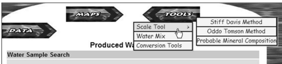
Figure 4. Tools included two scale calculation tools, a mineral composition tool, one to determine the composition of mixing of two waters, and unit conversion calculators.
