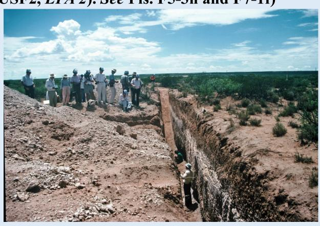
Pl. F7-1f (NM WRRI; 5/22/2007). Lower La Mesa surface exposure of Stage-IV petrocalcic soil in upper part of 1988 NMSU calcic-soil research trench shown in Pl. F7-1e.
