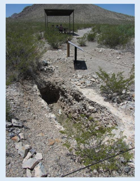
Pl. F6-1c (NM BMMR; **8/1982). Initial NMSU Soil-Moisture Research** Proj. excavation in piedmont-slope alluvial deposits. HSUs-PA/USF1 (LFA 5), with multiple buried soils, are exposed in 33-ft (10-m) trench. The photo site is in the SJB-Isaacks Ranch Subbasin; and the Mount Summerford (NE Doña Ana Mtns.) sedimentsource area is in the background. See Pl. F6-1d for trench detail
