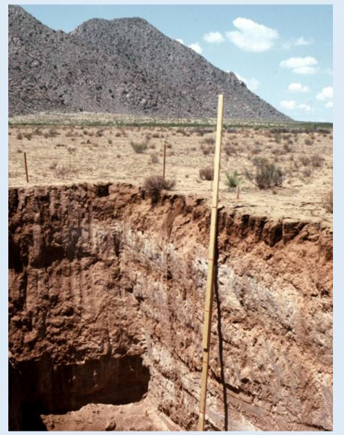
Pl. F6-1d (NMSU; 1983). Completed NMSU soil-moisture research excavation in piedmont-slope deposits derived from the Mount Summerford Area of the NE Doña Ana Mtns. About 33-ft (10-m) of HSUs-PA/USF1 (LFA 5), with multiple buried soils are exposed. *See* Pl. F6-1c for geomorphic setting
