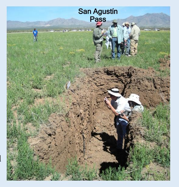
**Pl. F6-1f (NM** WRRI; 5/24/2007). Detail of Pl. F6-1e trench exposure of **Vertisol in Isaacks** Lake playa, with 2-m tape. Soil structure reflects high shrink-swell properties of clayrich (>60%  $<2\mu$ ) playa sediment
