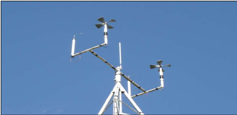
Figure 4: Setup of propellers and fine wire thermocouples
