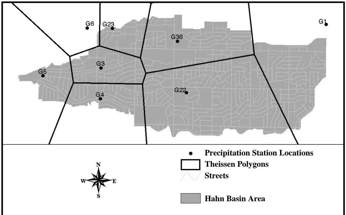
In this research, we identify the Thiessen polygons derived from these rain gage locations (see “Thiessen Polygons” in Figure5) and apply the rainfall amount recorded at each station in each 5-minute period uniformly to those cells within the Thiessen polygon surrounding each station. This method is only one of many different approaches that could be applied to this type of
