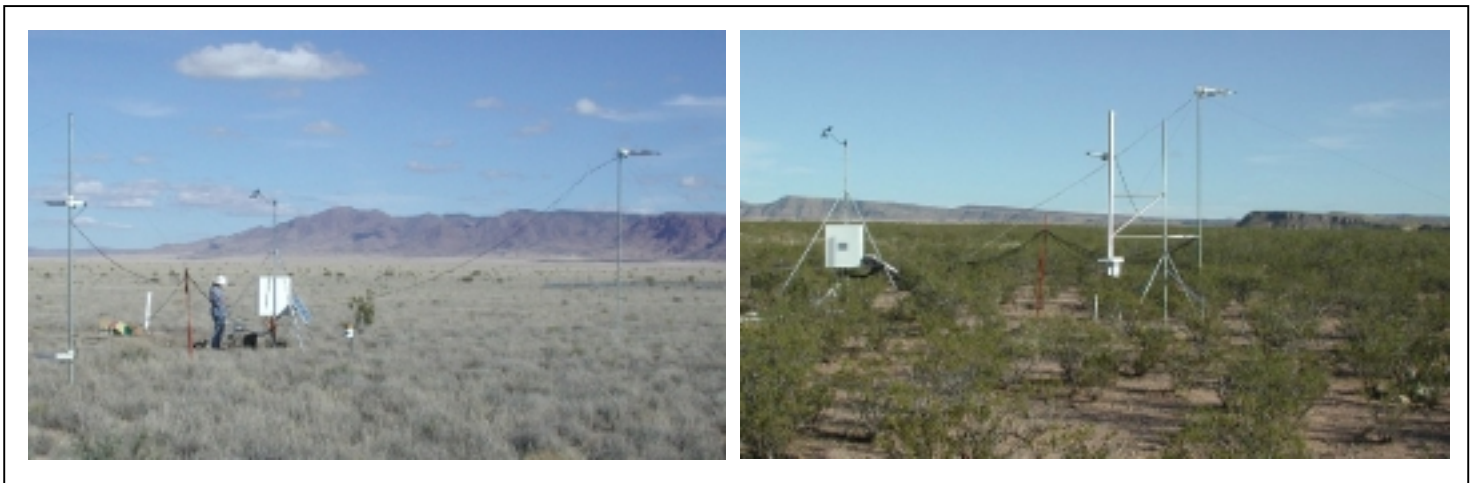
Figure 4. Grassland and shrubland micrometeorological stations. The temperature and humidity probes are on the left side of the photo in the grassland and at the center in the shrubland. The radiometers (net radiation, shortwave, and longwave) are on the right side of both photos. Ground heat flux and soil moisture are measured uphill of both stations, under both plant canopy and interspace.
