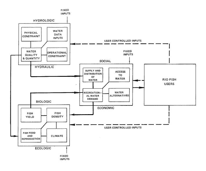
Figure 1. Schematic illustrating the interactions among the major model components and the model user. Solid lines indicate information flow whereas, dashed lines indicate user feedback control of model properties.
