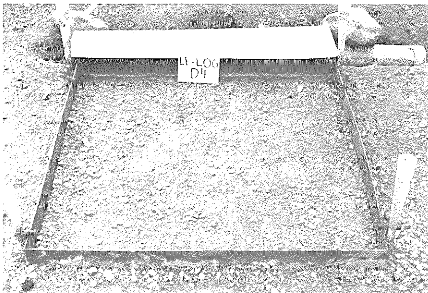
Figure 5. Installation in the Lincoln National Forest shows raingages and flashing cover
