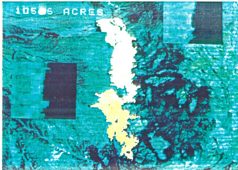
Figure 10. The initial surface area measurement obtained by the Band 7 density slice was 10,596 acres. The reported surface area by interpolation of published data was 12,122 acres. This represents a discrepancy of 13%.
