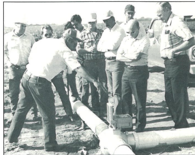
Farmers inspect a solar-powered surge irrigation valve during a field day on a farm near Deming. Surge valve irrigation helps smooth out the uneven distribution of water in furrows. (Photo by New Mexico Energy, Minerals and Natural Resources Department)
