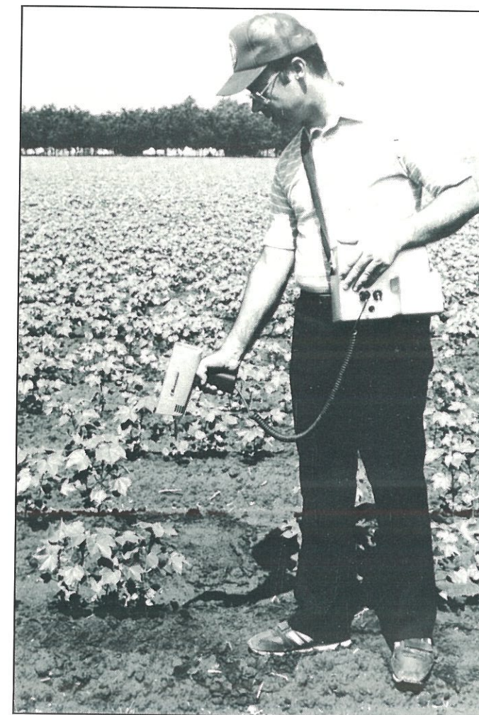
The infrared gun, when aimed at a plant, measures leaf and air temperatures, humidity and sunlight. From that, it determines if it is time to irrigate. Infrared guns can be cost-effective on very large farms. (Photo by New Mexico Water Resources Research Institute)
