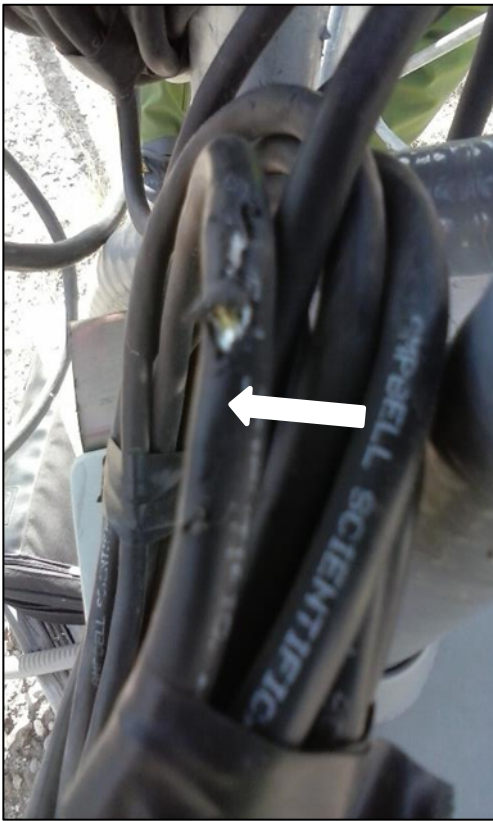
Figure 11. Left: Chew marks on sensor cable. Right: Spider webs on humidity and temperature sensor.
