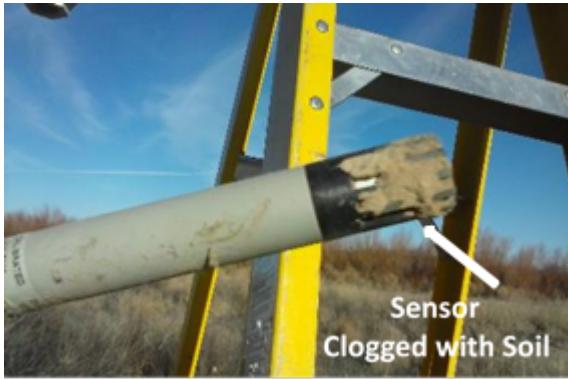
Figure 10. A Relative Humidity/Temperature sensor clogged with soil (left) and cleaned (right)
