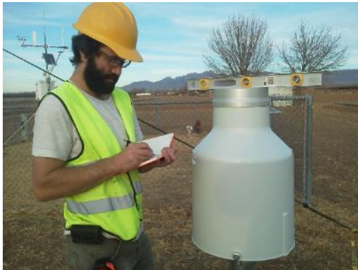
Figure 8. Garrett Gibson installing Pluvio rain gauge at Leyendecker
