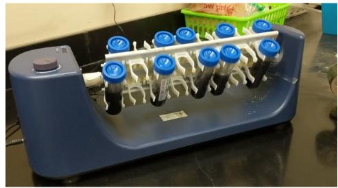
Figure 3. Batch mobility experiment procedure shown above. The image shows 50ml tubes on a rotator during the 5-hour time step of the experiment.
