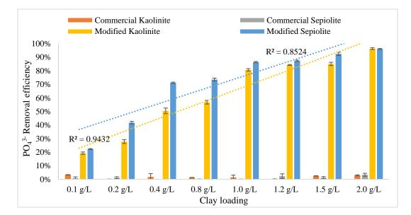
*Figure 2: Variation of phosphate removal efficiency with commercial and modified kaolinite and sepiolite clay loading*
