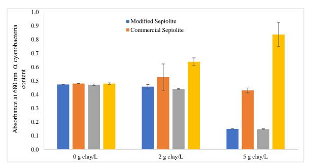
*Figure 1: Comparison of cyanobacteria removal by modified and unmodified sepiolite and kaolinite when packed inside a dialysis tube at different clay loadings*
