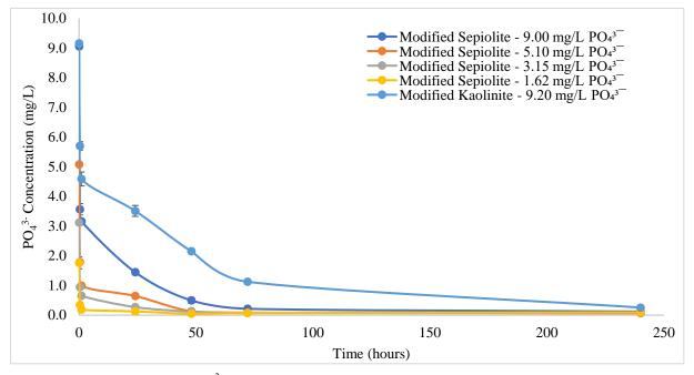
Figure 3: Variation of PO<sub>4</sub><sup>3-</sup> concentration over time for direct clay application of Modified Sepiolite and Modified Kaolinite for different initial PO<sub>4</sub><sup>3-</sup> concentrations
