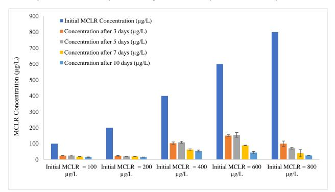
Figure 6: Variation of MCLR concentration over time for different initial MCLR Concentrations with modified sepiolite inside dialysis tubes
