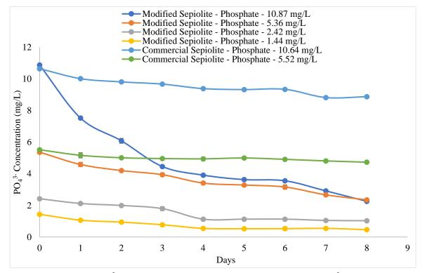
Figure 5: Variation of  $PO_4^{3-}$  concentration over time for different initial  $PO_4^{3-}$  concentrations with modified and unmodified sepiolite packed inside the dialysis tubes
