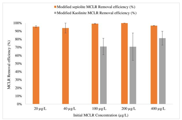
Figure 4: The variation of MCLR Removal by direct clay flocculation of modified sepiolite and kaolinite for different initial MCLR concentration
