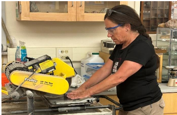
Dr. Lindline using rock saw to cut and prepare rock samples for testing (07/30/24). Photo c/o Mary Frances Bibb.
