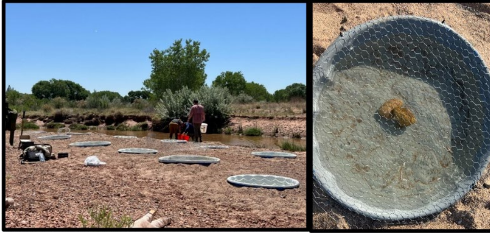
Figure 3. This composite image showcases two critical aspects of the Red Shiner mortality study. On the left, the setup is displayed with multiple pools of varying sizes bred within a sandy bar, simulating isolated aquatic environments. On the right, a close-up view of one such pool is provided, featuring the predator control wire mesh cover in place., which is utilized to assess the impact of predation on fish survival rates within the experimental framework.
