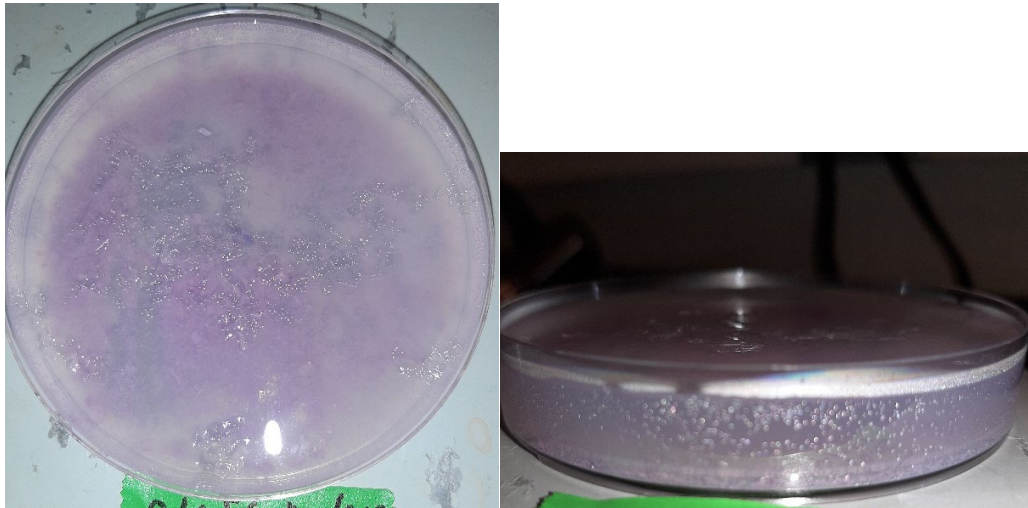
Figure 22: Presence of air bubbles in the reaction solution during UV irradiation
