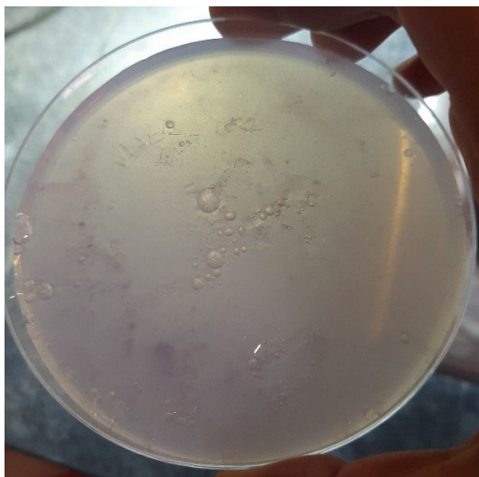
Figure 23: Bubbles present in the bottom surface of the floating PET particles
