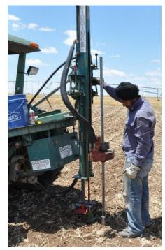
**Figure 3.** Installation of neutron access tubes in the study area.
