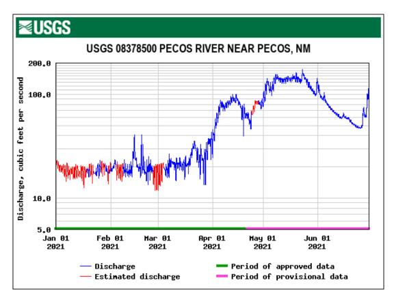
Figure 3. Discharge along the Pecos River at USGS gaging station 08378500 near Pecos, NM. For the project sampling dates, discharge averaged 17.8 ft<sup>3</sup>/sec on January 18<sup>th</sup>, 21.3 ft<sup>3</sup>/sec on March 17<sup>th</sup>, 138 ft<sup>3</sup>/sec on May 13<sup>th</sup>, and 71.4 ft<sup>3</sup>/sec on June 29<sup>th</sup>. Data from USGS Current Water Data for New Mexico (URL: <u>https://waterdata.usgs.gov/nm/nwis/rt</u>?).
