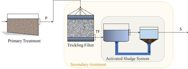
Fig 1. The diagram of sampling points (P, TF, and S)
