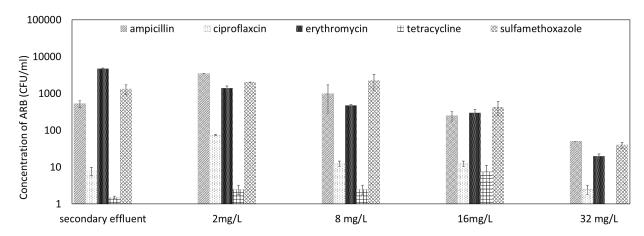
Fig 4. The concentration of ARB after different concentration of NaClO treated
