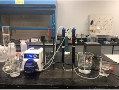
Fig 1. The GAC column setting for ARB removal
