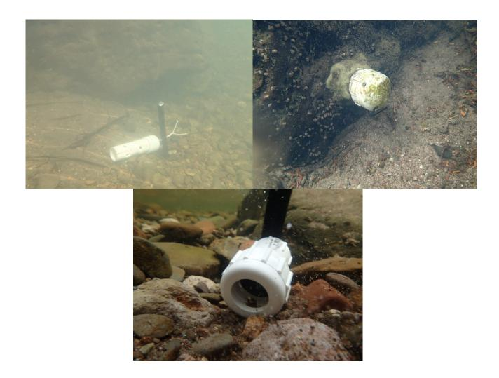
**Figure 1:** Types of temperature loggers used include ProV2 (top left), Tidbit v2 (top right), and the adapted Stream Temperature, Intermittency, and Conductivity (STIC) logger (bottom). ProV2 and STIC models are anchored with three foot framing stake and ten gauge wire, Tidbit v2 model is affixed to a permanent stream structure using two-part waterproof epoxy.
