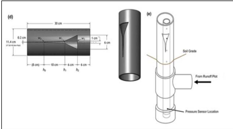
Figure 3: UBeTube original schematic.
