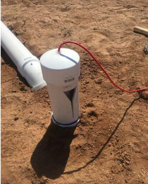
**Figure 7: UBeTube device installed.**
