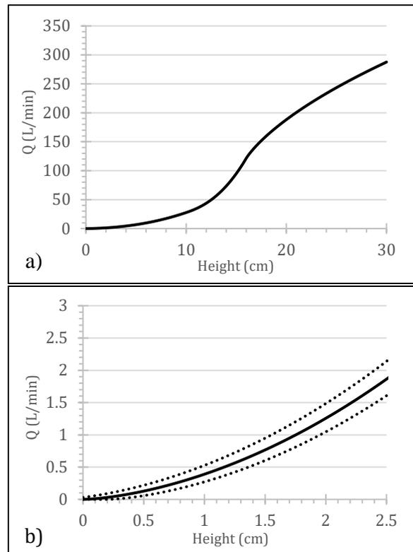
Figure 5: a) Rating curve for UBeTube configuration with correction coefficient of 0.95, and b) Detail of curve at low flows. Dotted lines indicate 2mm resolution of sensors.
